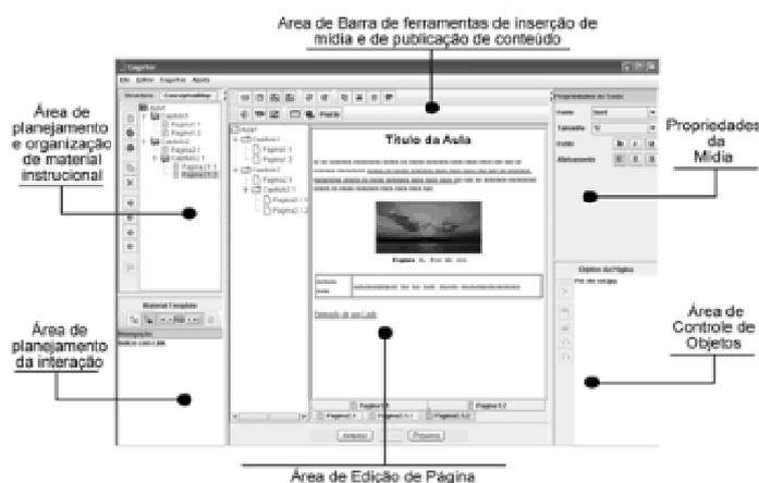
Figura 2 – Interface principal da ferramenta Cognitor
