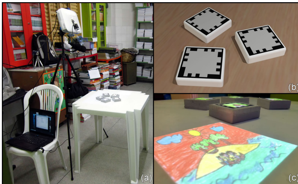
Figure 1. ARBlocks setup is shown on the left (a). The blocks, on the top right (b), were designed especially for children and have an empty area in the middle where the virtual content will be displayed, as seen in the bottom right (c). It is also possible to use the table as a projection and interaction area.
