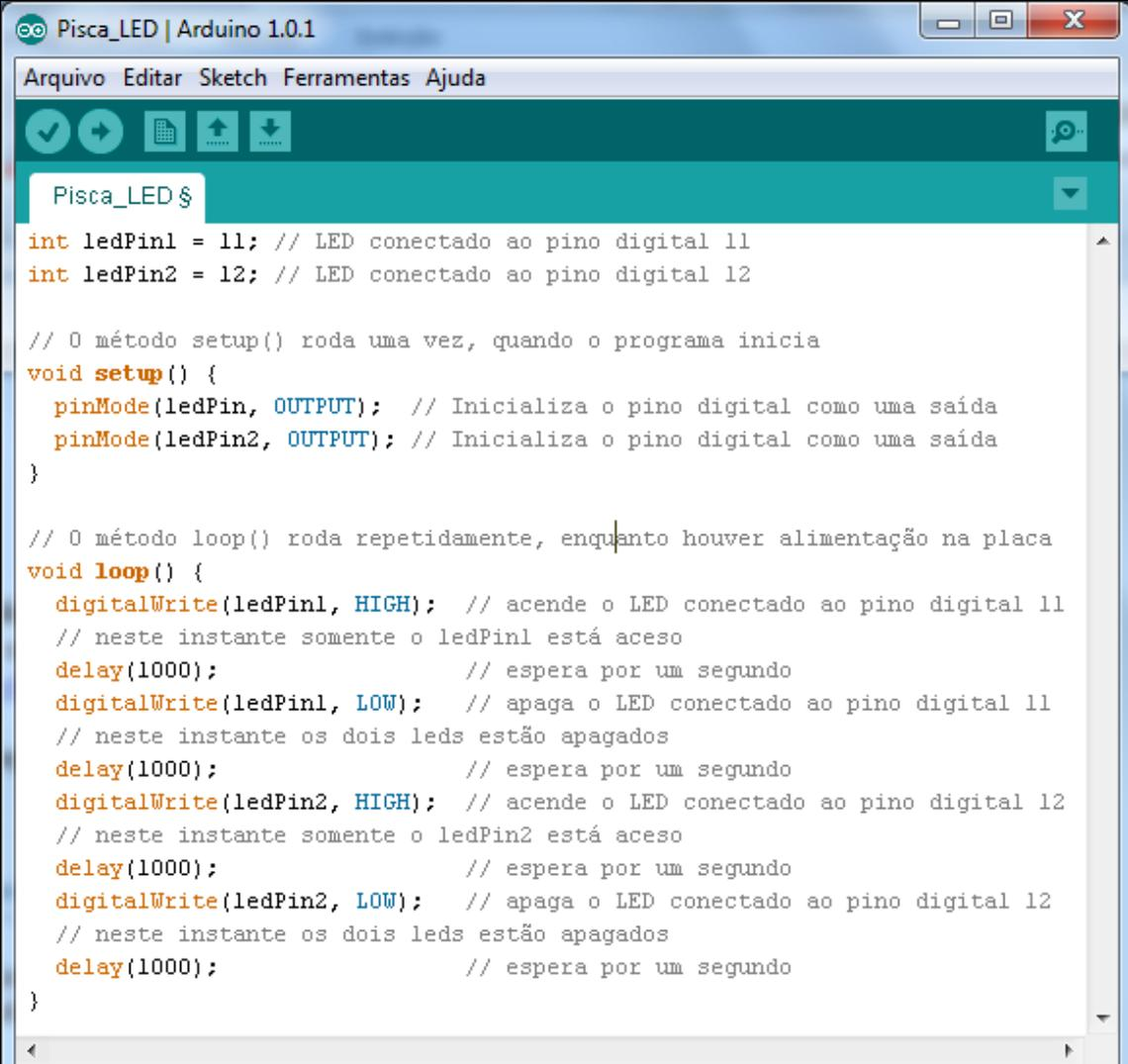
The image shows a screenshot of the Arduino IDE interface. The window title is 'Pisca\_LED | Arduino 1.0.1'. The menu bar includes 'Arquivo', 'Editar', 'Sketch', 'Ferramentas', and 'Ajuda'. Below the menu bar is a toolbar with icons for saving, running, uploading, and downloading. The main text area contains the following C++ code:
